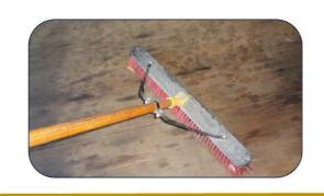
B Check floor for nails or screws protruding up from container floor using the back surface of the 24" shop broom.
