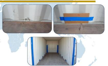
Corner lashing rings will need to be protected using 2 x fluted plastic
