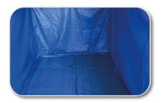
Confirm flexitank is positioned equally inside container before product flow is started.
