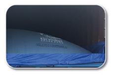
Flexitank will continue to rise until the flow meter, scale or automated system indicates the load amount has been reached.
