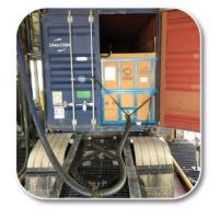
If possible load line should be supported on the chassis to relieve excess weight from valve.
