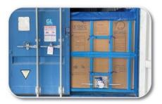
Right hand door will need to be open and secured to the side. Check bulkhead to confirm it's not damaged and it's fully seated into recess.
