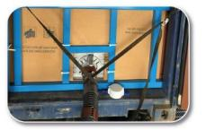
Option 1: Clear load line into flexitank via air.
