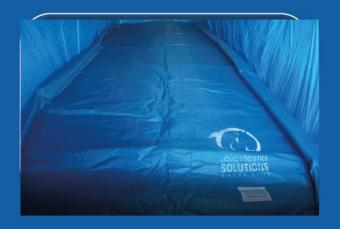
During discharge flexitank will collapse in the middle leaving side last to fall down.
