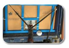
Adjustment of support strap after 10 minutes of product loading might be necessary.
